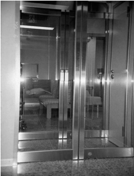
FIGURE 5.6 Entrance of a clean room for CS patients with positive air pressure control to prevent entry of chemicals pollution from the outside. The room is also shielded against electromagnetic waves.
